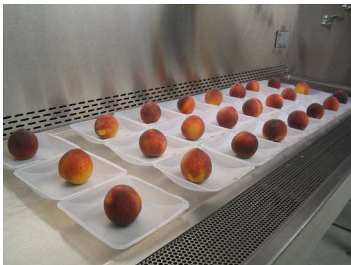
Figure 3.1. Inoculated peaches drying under a biosafety hood for 20 – 22 h at 22 \pm 2 °C prior to treatment with gaseous ClO_2 .
